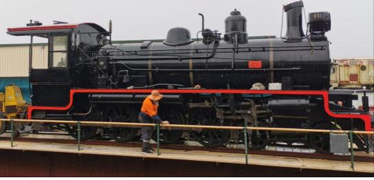
Since the last news update, our C17 locomotive number 971, has had the refurbished wheel sets and axle boxes replaced and will now have the final bits and pieces re-fitted ready for a long awaited return to duties. Well done the hard working engine shed team!
