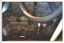
The Flier is a diesel - mechanical vehicle, meaning the 102hp Garner diesel engine drives directly to the wheels, rather than via electric or hydraulic motors, as is the case with most locomotives.
